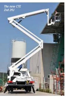
The company will also show its new 29 metre ZED 29 J articulated truck mounted lift with dual parallelogram sigma riser, three section top boom and articulating jib. The stowed unit has a compact eight metres overall length, a GVW of 10.5 tonnes and offers up to 15 metres of outreach.
