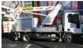
This 18 metre Palfinger P180 was spotted on the Palfinger stand which expands the bottom end of its Premium Class range of machine's on a 7.5 tonne chassis. The platform has plenty of carrying capacity.
