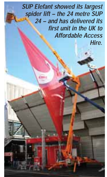
The double articulated CMC 240TB has a 24 metre working height and 11.3 metre outreach on a 3.5 metre chassis.
