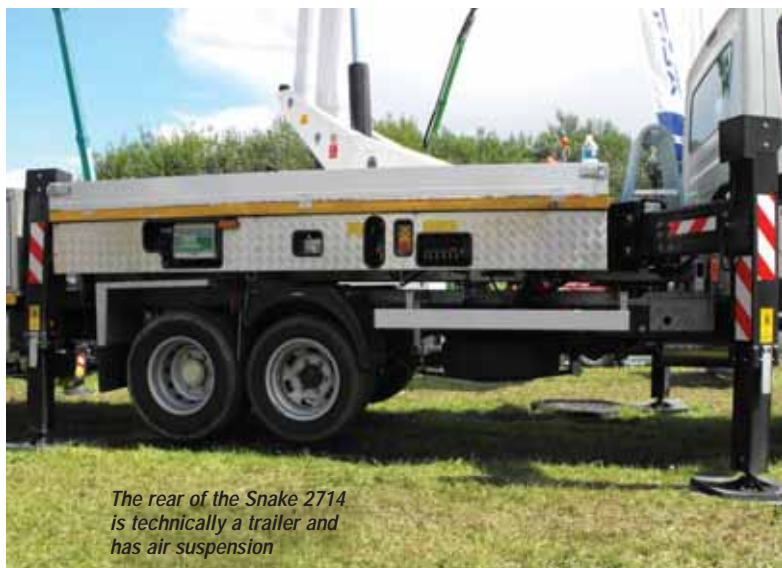
The 2714 is essentially made up of a chassis cab with fifth wheel and a trailer with lift.
