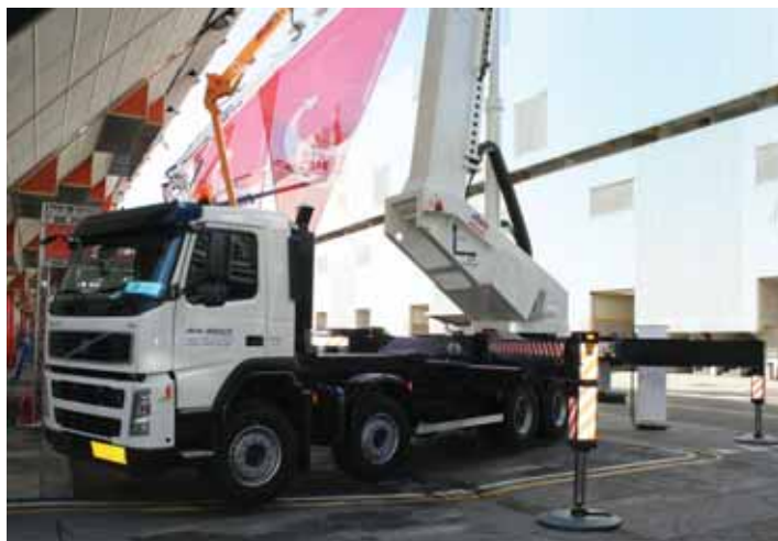
Not quite the tallest platform at the show, Barin showed off its 73 metre AP73-35J2 with 35 metre outreach.
