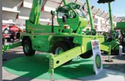
The new GSR E210PX is lower and shorter than other GSR PX models and offers 10.3 metres outreach and 10% slope levelling.
