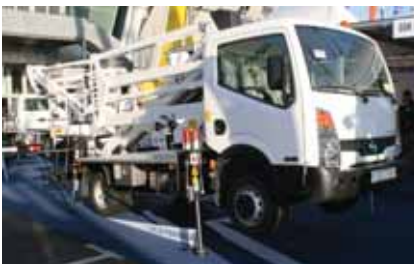
The new GSR E210PX is lower and shorter than other GSR PX models and offers 10.3 metres outreach and 10% slope levelling.
