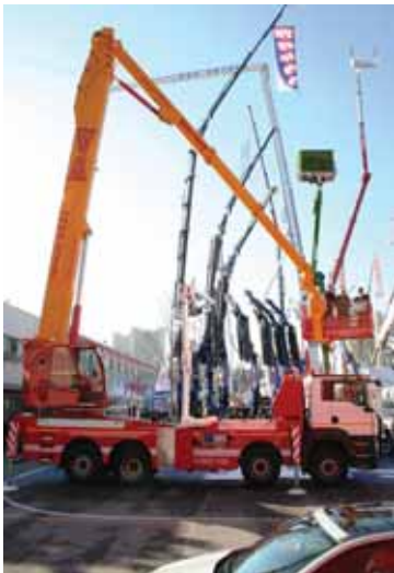
Oil&Steel showed its new 60 metre Eagle 6035 - it has a 35 metre outreach, 360 degree platform rotation with 500kg capacity.
