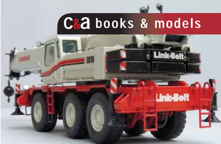
Counterweight slabs are removable
