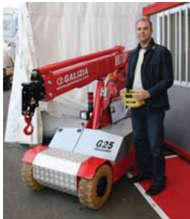
Fabio Galizia showed off his new remote controlled G25. By removing the handle controls from its G20 and adding more counterweight, the capacity has been upped to 2.5 tonnes. The company says it should have its new range of 'F200 type' machines – from 12 to 35 tonnes – by next Autumn.
