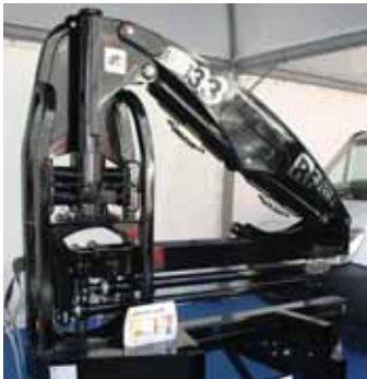
First showing for the Italian RF333.A1 New Concept Crane. Designed by Romano Ferrari for mounting behind the cab of an Iveco Daily it has a 2.5 tonne maximum capacity and six metre reach.
