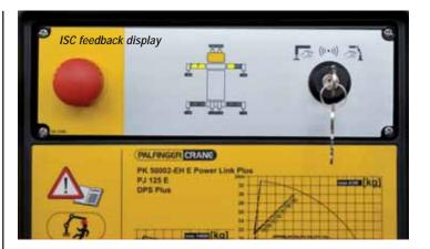
hydraulic rated capacity limiting device. The system allows crane operation in a single configuration i.e. when all four outriggers are fully extended and in contact with the ground. The FSC-M is a mid-range solution for cranes ranging from the F22A to F260DXP used in conjunction with the FX500 RCL device. In this case, the system allows the crane to operate in two working configurations firstly, beams fully retracted with jacks down and secondly with outriggers
