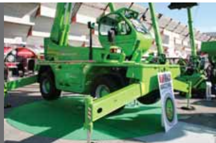
The new GSR E210PX is lower and shorter than other GSR PX models and offers 10.3 metres outreach and 10% slope levelling.
