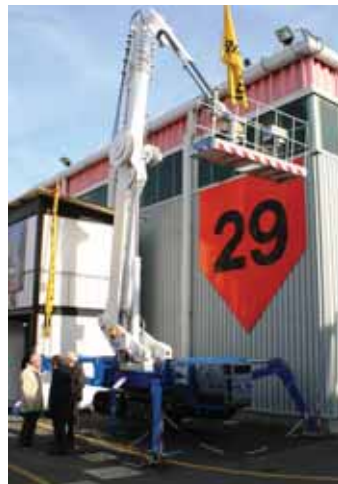
Palazzani showed off its expanding range of spider platforms including this 42 metre XTJ42.
