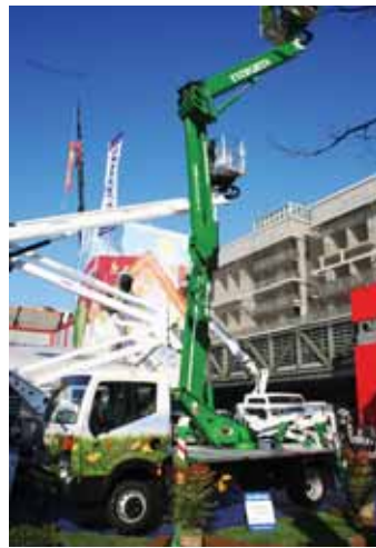
Oil&Steel's 20 metre 'green' Snake 2010 Compact incorporates many hydraulic system changes to accommodate the use of biodegradable fluids.
