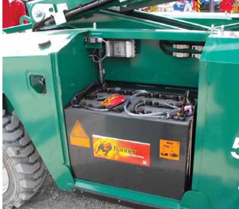
Full traction battery packs are being used more widely on aerial lifts.
