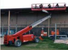
outreach (14,20 m) and rotation (180) of a telescopic boom lift For hire at:
