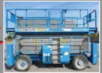
Genie GS 5390 Diesel scissor lift 18m/680kg - 2005/6/8
