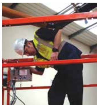
The idea is that if an operator is pushed down on the controller his forearm will activate the system.
