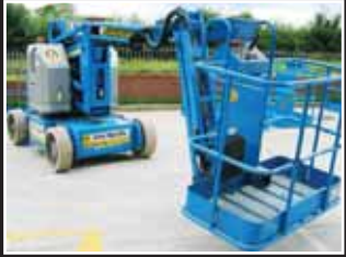
Genie Z-34/22N Articulated boom 12.50m - 2005/6
