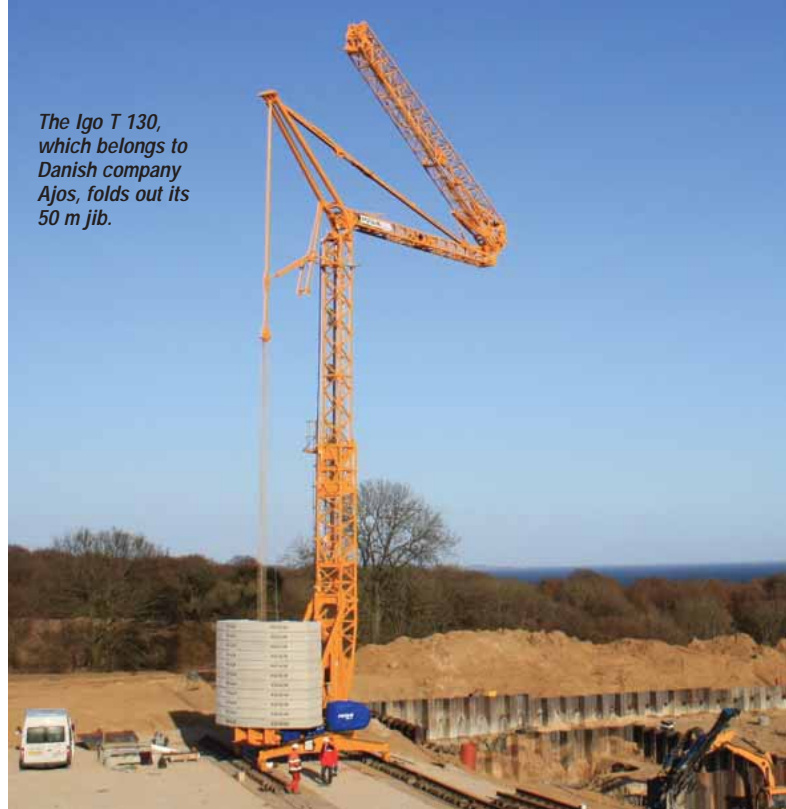
The Igo T 130 is easy to transport and can be ready to work in less than four hours
