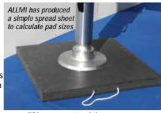
calculation of the lorry loader's gross lifting moment and the forces exerted through the stabiliser legs.
