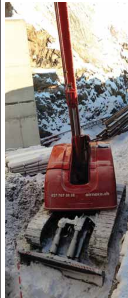
The Giraf Track's compact dimensions allowed it to move in very close to the lift.
