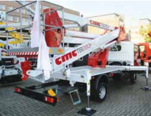
One of the 'must see' exhibits - the TB260 a 26 metre articulated platform on a 3,500kg chassis from CMC. Also on the stand was Jonathan Wiseman who announced he had joined CMC from CTE to look after sales and support in the UK and Ireland.
