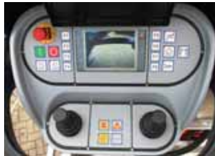
The new Palfinger control panel can mimic other manufacturers' controls.
