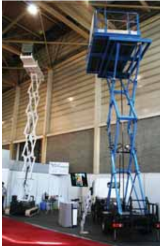
Mavel Tech's new 9.7 metre Airlift SF10 3.5 tonne truck mounted scissor with 500mm platform side extension was first seen at Bauma but is now in production. The company also manufactures narrow wheeled and tracked scissors to 20 metres.
