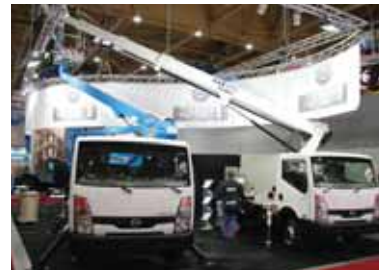
Isoli was supposed to launch two new articulated booms on short wheelbase 3.5 tonne Nissan Cabstar chassis but unfortunately the 23 metre PNT 230 didn't quite make it although the 20.5 metre PNT205LNX - a deluxe PNT205S with 230kg platform capacity - did.
