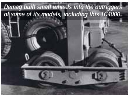
An outrigger bogie from the 1960s?
