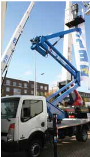
CTE brought along its new 20 metre ZED 20 CSH - the S indicating a higher working capacity of 250kg compared to its ZED 20 CH model.
