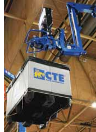
CTE showed this quick-release winch attachment for its Tracess spider lifts that can lift 250kg.
