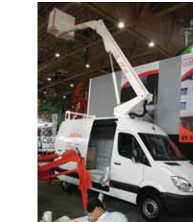
Italian platform manufacturer Easylift showed this new, 13 metre EV130 van mounted platform.
