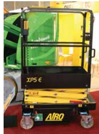
The new 2.55 metre platform height XP5 E is one of two new push around scissor lifts from Airo. The other is the similarly sized but 3.34 metre platform height, XLP5 E. Also new were two new battery powered articulated industrial boom lifts the A12JE and the A15JE.
