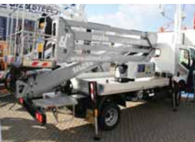
Oil&Steel launched its new 23 metre Snake 2311 Compact REL mounted on a 3.5 tonne chassis and in-board outriggers aimed at the rental sector.
