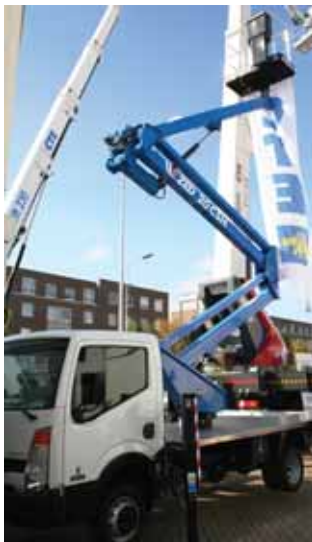
CTE brought along its new 20 metre ZED 20 CSH - the S indicating a higher working capacity of 250kg compared to its ZED 20 CH model.
