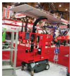
Shown for the first time in Europe, Bravi's dry wall/plaster board handling device for its Leonardo lift.
