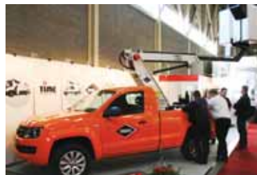
Time Versalift launched the LT-23/30-TB Electric platform, the first based on the VW Amarok 4x4. Working heights are 9.2 metres and 11.2 metres with 4.2 metres outreach.
