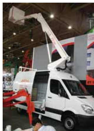
Italian platform manufacturer Easylift showed this new, 13 metre EV130 van mounted platform.
