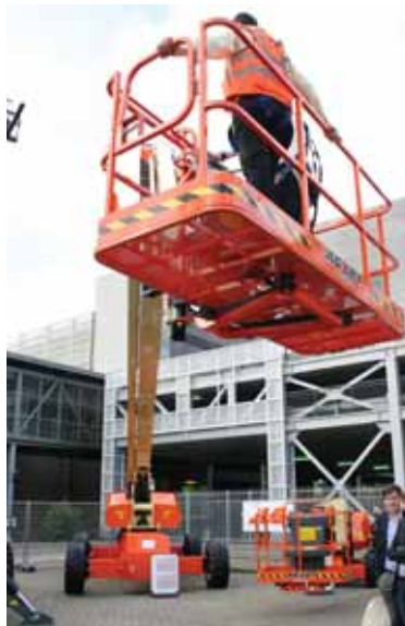
JLG exhibited the world's largest self-propelled boom - the 150ft platform height /47 metre working height JLG 1500SJ - on its outside stand. Visitors could see the recently launched 340AJ and the new smaller Toucan 8E mast boom.
