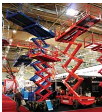
As usual the Holland Lift stand was crammed full of exhibits, including its new 39ft platform height/14 metre working height compact Ecostar and 86ft/28 metre N265-EL13 narrow aisle heavy duty scissor.
