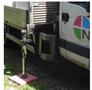
The mat on the unloading side on the dry lawn. At the rear a mat was used on interlocking blocks - not necessary but still good practice.
