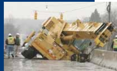
Being aware of ground conditions also applies to equipment working free on wheels
