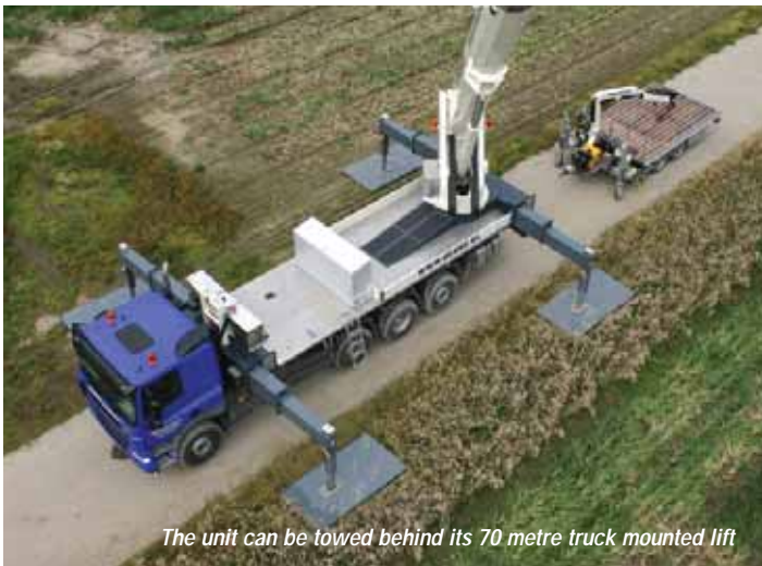
A good example of a steel mat with sand to provide a good base.
