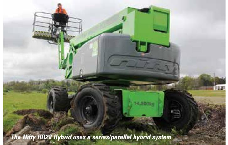
The Nifty HR28 Hybrid uses a series/parallel hybrid system
