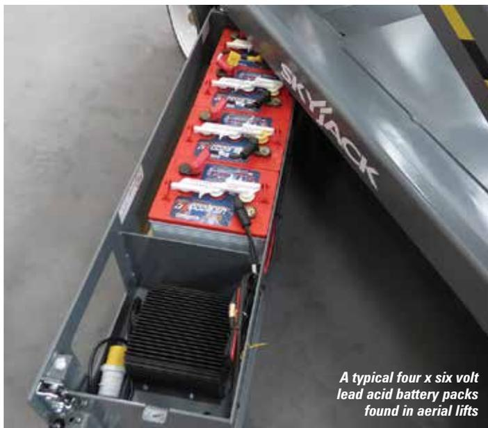
A typical four x six volt lead acid battery packs found in aerial lifts
