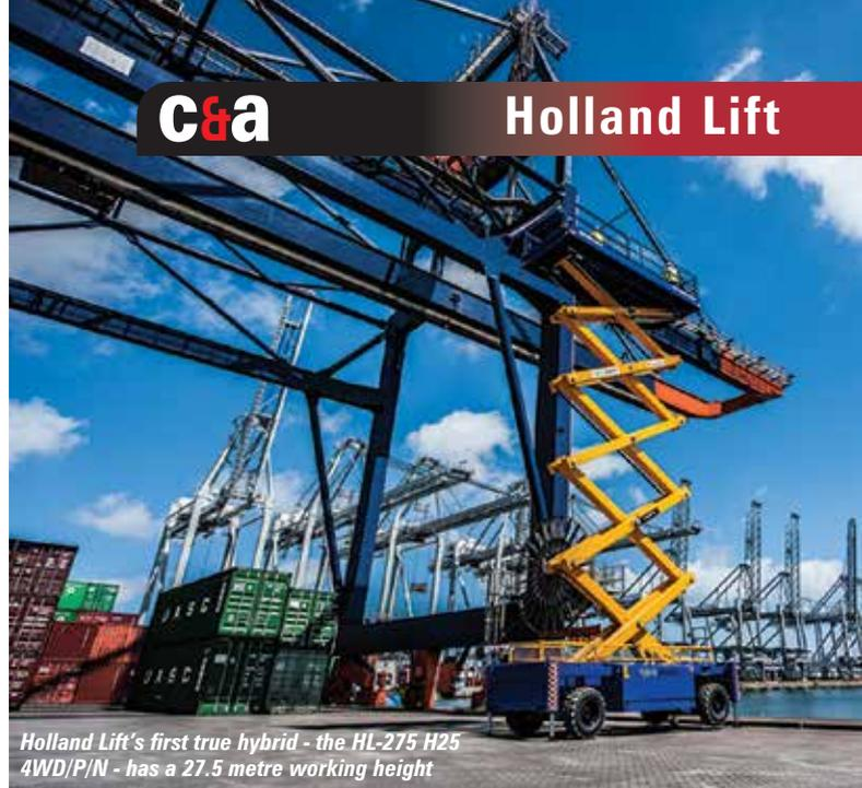
Holland Lift's first true hybrid - the HL-275 H25 4WD/P/N - has a 27.5 metre working height
