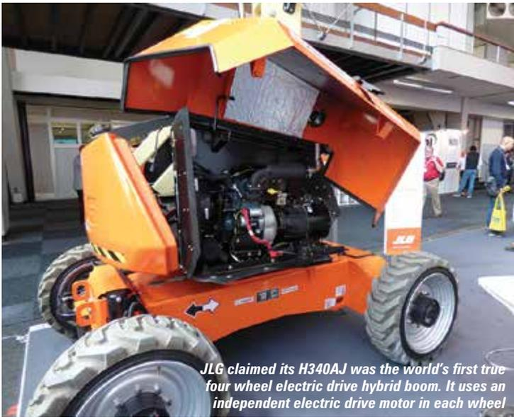
*JLG claimed its H340AJ was the world's first true four wheel electric drive hybrid boom. It uses an independent electric drive motor in each wheel*
