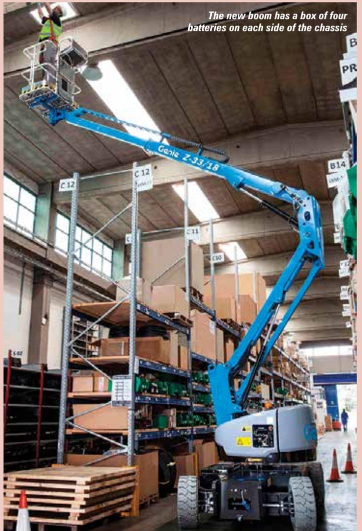
The new boom has a box of four batteries on each side of the chassis
