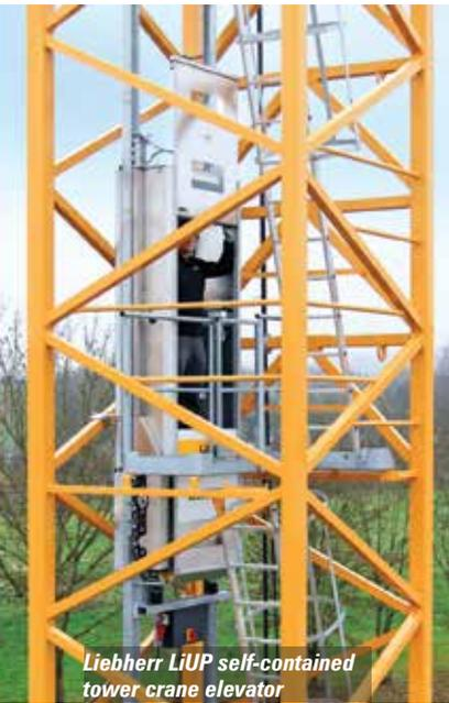
Liebherr LiUP self-contained tower crane elevator
