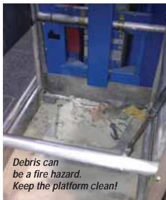
should do the pre-start inspections and daily checks. This would help identify any debris, leaks, spills, damaged cables and wiring, or other fire hazards, and allow preventive action to be taken."
