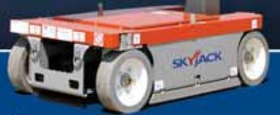
Skyjack's new SJ12 self propelled vertical mast lift provides a compact footprint and superior maneuverability. When operating in tight workspaces, a high degree steer angle allows for maximum functionality and flexibility by offering zero inside turning radius. The SJ 12 also features a 20" traversing platform, providing increased access and the ability to reach over potential obstacles. A unique slide away platform provides easy access to components, when raised or in the stowed position.
