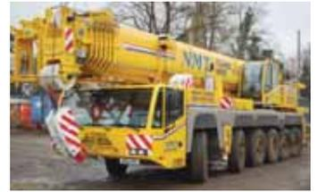
NMT's new six axle Terex AC200-1P can travel with up to 25 tonnes of counterweight along with all its tackle and steel outrigger mats.
