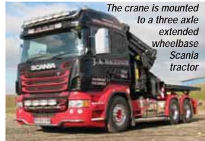
The crane is mounted to a three axle extended wheelbase Scania tractor
