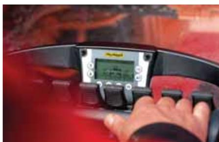
Both main control station and remote controller displays show percentage of extension for each outrigger
