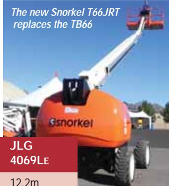
The company says that at 1.37 metres, the T66JRT offers by far the best inside turning radius of any two-wheel steer boom in its class. The unit is also compact with an 8.5 metre overall length and 2.5 metres overall height.
