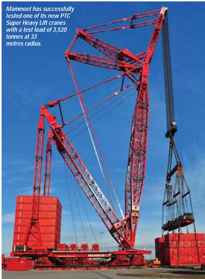
International lifting specialist Mammoet has successfully tested one of its new PTC Super Heavy Lift cranes with a test load of 3,520 tonnes at 33 metres radius.
