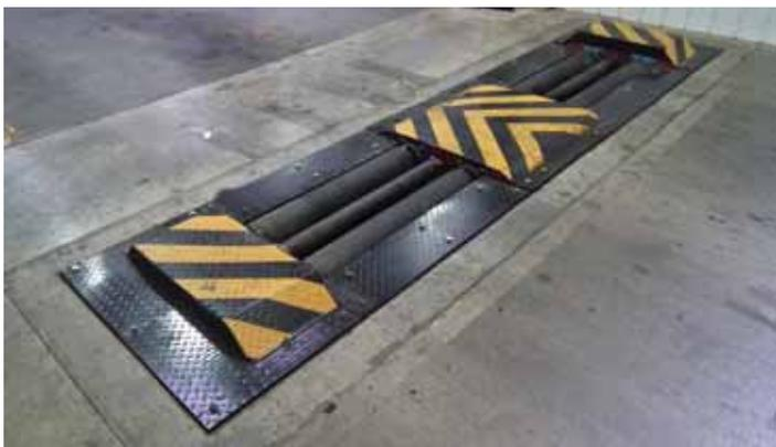
The rollers can be adjusted for vehicles with overall widths from three metres down to 2.4 metres
