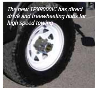
The new TPX9000IC has direct drive and freewheeling hubs for high speed towing
