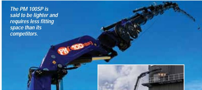
highest grade steels we have gained considerable weight reduction, while the new octagonal boom profile increases the loading performance and improves rigidity. Less flex means more stability and increased accuracy."
