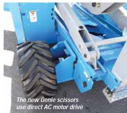
The new Genie scissors use direct AC motor drive
