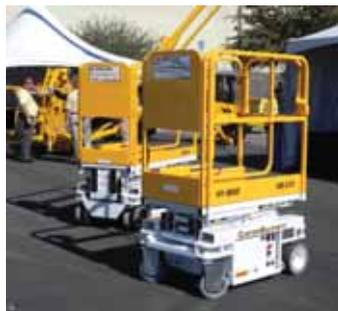
*Custom Equipment with its 8 and 10ft low level self-propelled scissors.*
