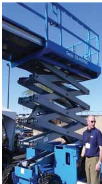
Senior product manager Jeff Weido with the GS3369DC, the full 1.5 metre deck extension will be blocked at 1.17m on CE models
