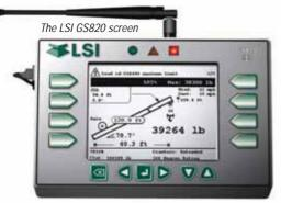
readable screen, on-board data logger and the ability to upload load charts via the USB port or download the logged data via USB stick. The unit provides a simple readout of all crane geometries, working load limit, actual load, selected chart/counterweights, wind speed, alarms and system faults.
