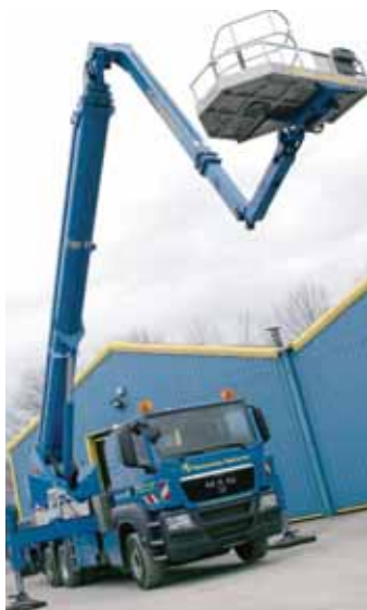
Larger trucks can be fitted with a specific TV cage.
