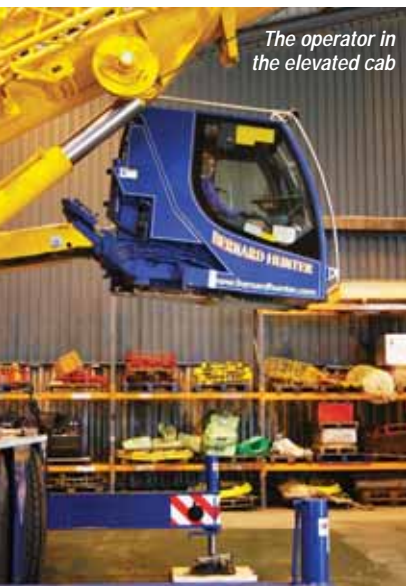
Elevating the cab on the LTC 1045 gives the operator a vastly improved view of the lift
