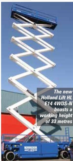
The new Holland Lift HL E14 4WDS-N boasts a working height of 33 metres
