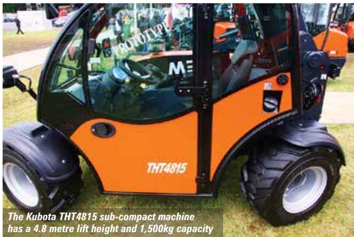
The Kubota THT4815 sub-compact machine has a 4.8 metre lift height and 1,500kg capacity
