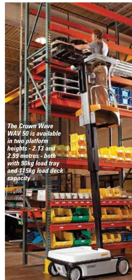
*The Crown Wave WAV 50 is available in two platform heights - 2.13 and 2.99 metres - both with 90kg load tray and 115kg load deck capacity*
