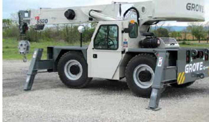
will travel with its maximum 16 tonne load at 800mm from its front bumper, as opposed to the 18 tonne Yardboss YB5520 that can only manage six tonnes.
