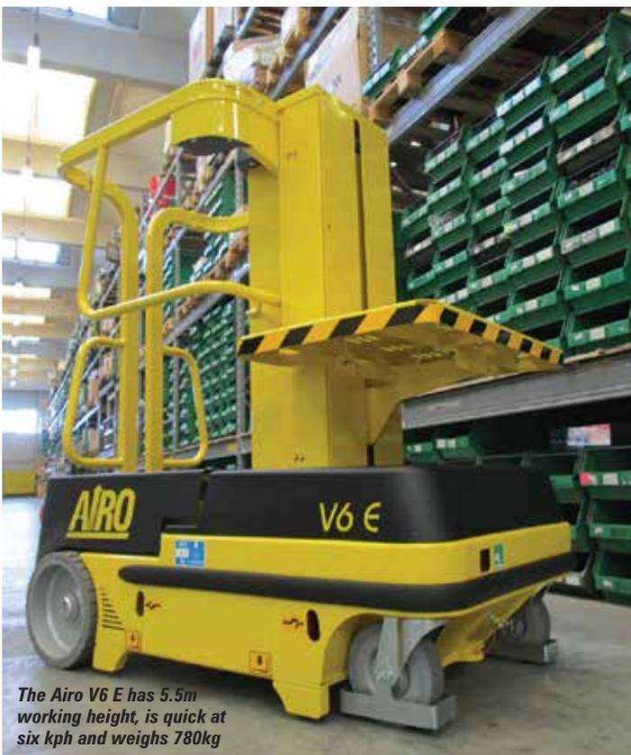
*The Airo V6 E has 5.5m working height, is quick at six kph and weighs 780kg*
