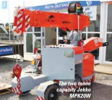
The two tonne capacity Jekko MPK20W
