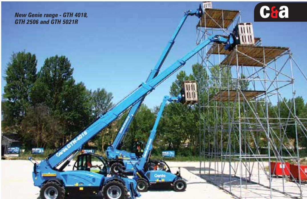
of its GTH range. The new range of six machines is aimed squarely at the rental market, and focused on end users in the construction, waste handling, recycling, industrial and logistics sectors. All models - both fixed frame and 360 degree - are designed to be simple, rugged and easy to run. The range includes the fixed boom compact six metre/2.5 tonne GTH 2506, and 14 or 18 metre/four tonne GTH 4014 and GTH 4018 as well as three rotating models - the GTH 4016R, GTH 4018R and GTH 5021R.
