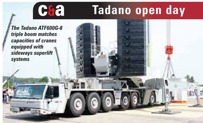
The Tadano ATF600G-8 triple boom matches capacities of cranes equipped with sideways superlift systems
