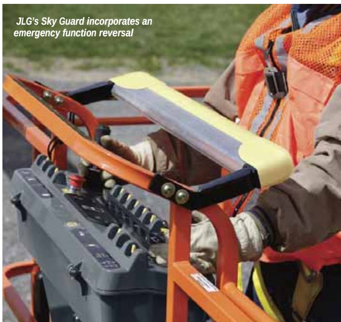
The rubber switch can be activated by pressure from any direction
