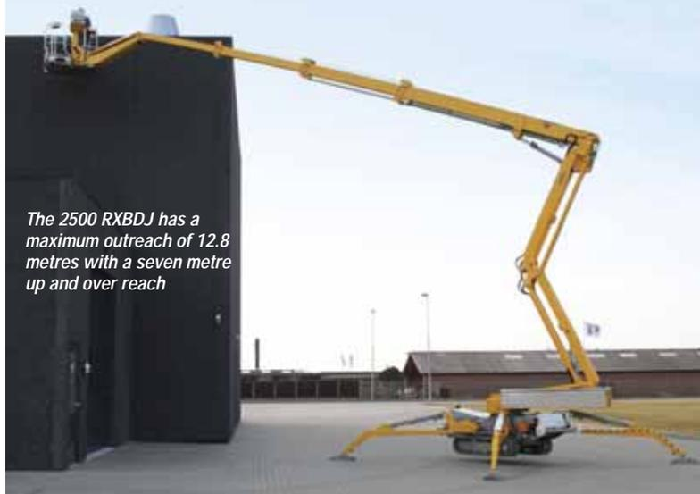
The 2500 RXBDJ has a maximum outreach of 12.8 metres with a seven metre up and over reach
