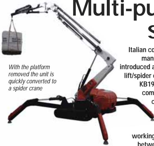
With the platform removed the unit is quickly converted to a spider crane
