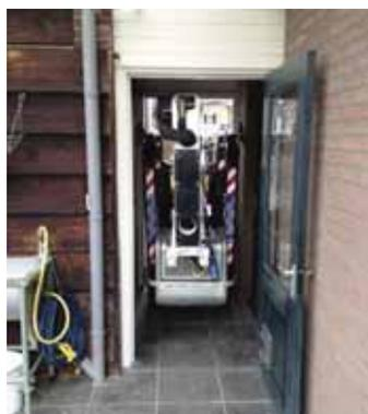
Hoogwerker Centrum realised that the only platform able to fit was a compact tracked spider lift and selected an Oil&Steel Octopussy Classic 1402.
