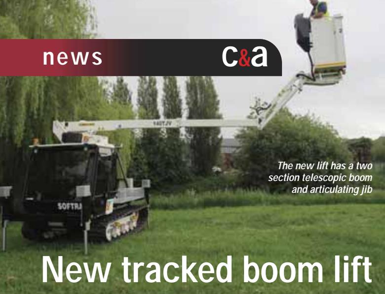
The new lift has a two section telescopic boom and articulating jib
