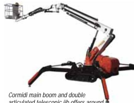
Cormidi main boom and double articulated telescopic jib offers around seven metres of horizontal outreach at an up and over height of around 14 metres.
