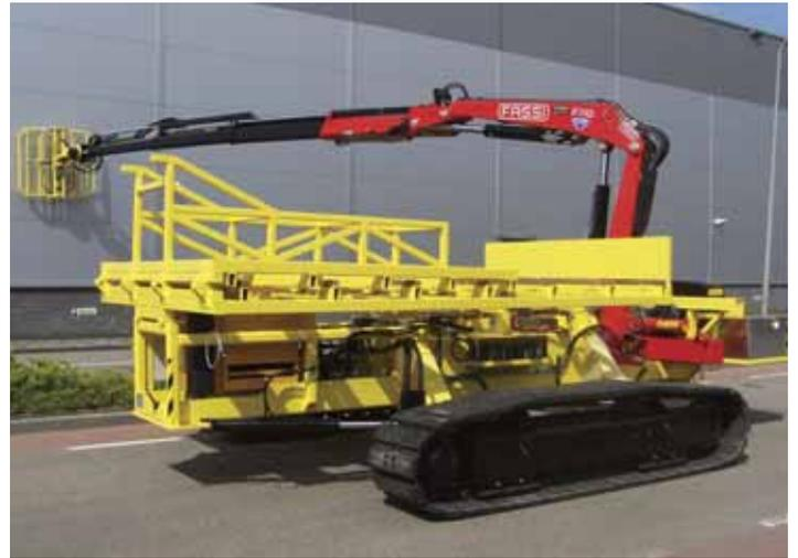
Dutch aerial lift manufacturer Omega Platforms has built two track mounted cranes for AG group of Norway for tunnel work. The first unit, designed and built at the end of last year, has proved its worth picking steel mesh rebar sheets from an on-board stack and placing them into the roof and walls of tunnels. The second unit has just been delivered.
