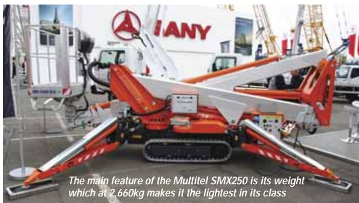
The main feature of the Multitel SMX250 is its weight which at 2,660kg makes it the lightest in its class
