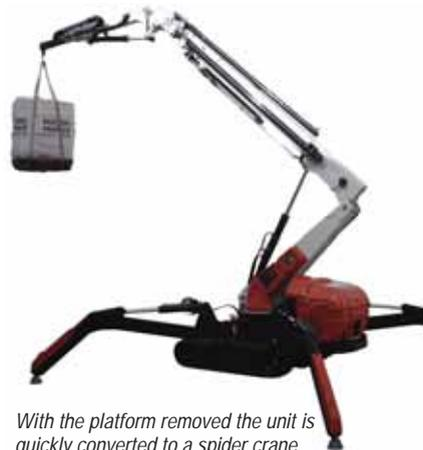
With the platform removed the unit is quickly converted to a spider crane.
