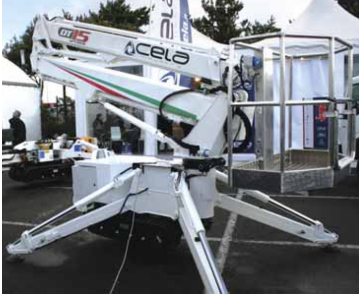
The DT15 is unusual in that it features a two stage highly versatile outrigger system and is lightweight at just 1,550kg.
