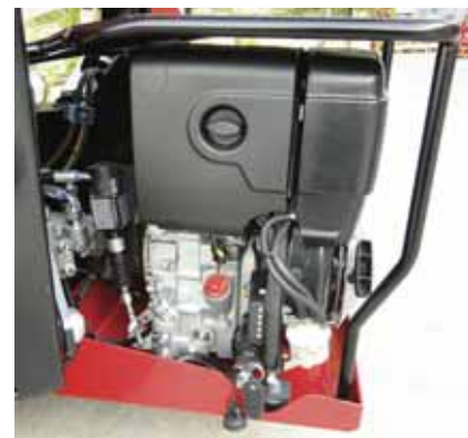
From 2012 Hinowa is introducing a three step automatic setting with speeds of 1,800, 2,200 and 3,600 rpm depending on function demand.
