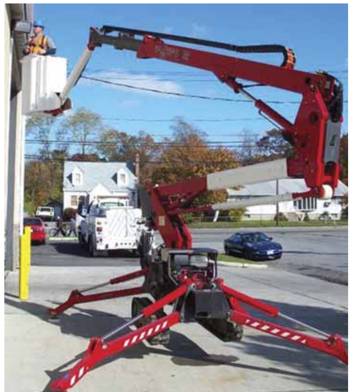
The 17 metre PB18.90.46 is fully insulated to 46KV with special fibreglass sections in the riser and levelling linkage as well as the jib.
