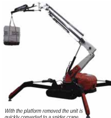
Cormidi main boom and double articulated telescopic jib offers around seven metres of horizontal outreach at an up and over height of around 14 metres.
