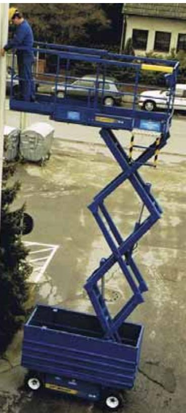
The idea of an electric scissor lift that can handle gravel and softer ground has been around for more than two decades - one such machine was the UpRight XL24 from the late 80s and early 90s.
