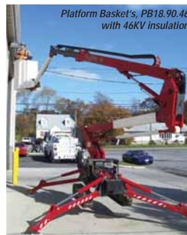
Platform Basket's, PB18.90.46 with 46KV insulation
