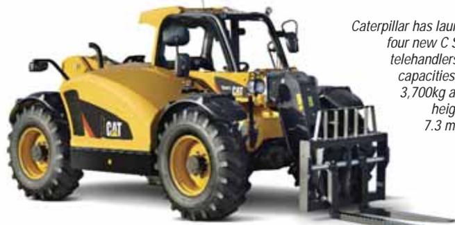
Caterpillar has launched four new C Series telehandlers with capacities up to 3,700kg and lift heights to 7.3 metres.
