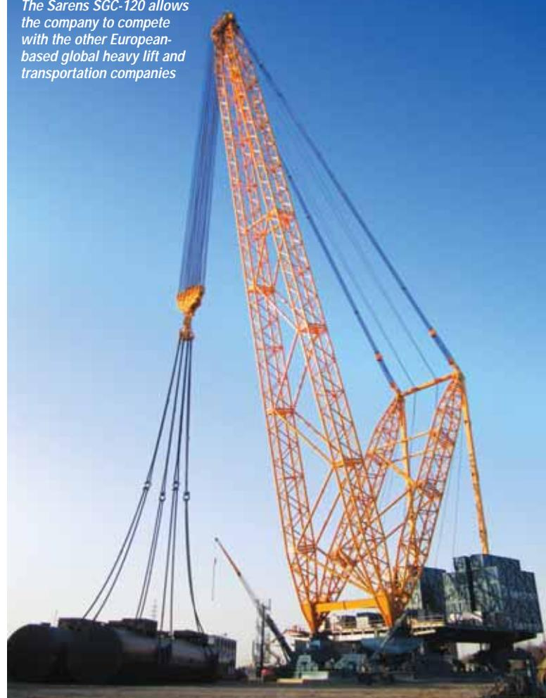
it semi-rigged this can be reduced to one day, but there are associated risks in moving such a crane including not putting down enough load spreading mats, the quality of the access roads which need to be wider and more stable than for trucks etc. There is always a cost factor and corners can be cut to reduce the time or costs," he says.
