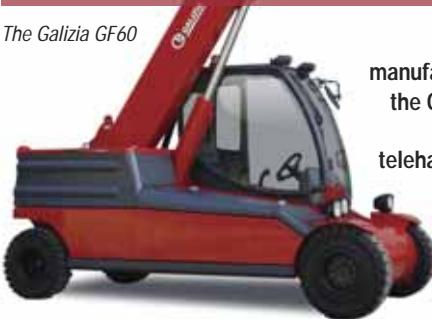
Italian pick & carry crane manufacturer Galizia has launched the GF60, a new six tonne crane based on its innovative telehandler/crane/platform Multis 636. The GF60 has a longer three section boom, with 7.5 metres under hook height.
