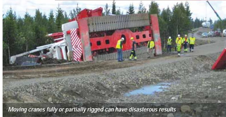
Moving cranes fully or partially rigged can have disastrous results
