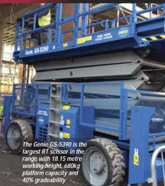
The Genie GS-5390 is the largest RT scissor in the range with 18.15 metre working height, 680kg platform capacity and 40% gradeability
