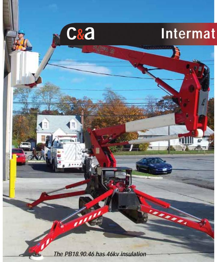
The PB18.90.46 has 46kv insulation
