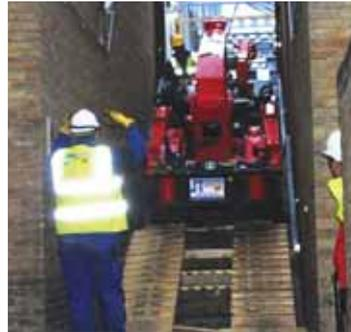
development has resulted in a four model range, two of which are now CE marked for the European market. The CE cranes are the 2.8 tonne CR285D, which weighs 1,750kg and boasts an 8.9 metre main boom and the significantly larger CR335D which, although it is rated at 2.98 tonnes, is significantly larger, weighing 3,760kg and featuring a 12.5 metre main boom.
