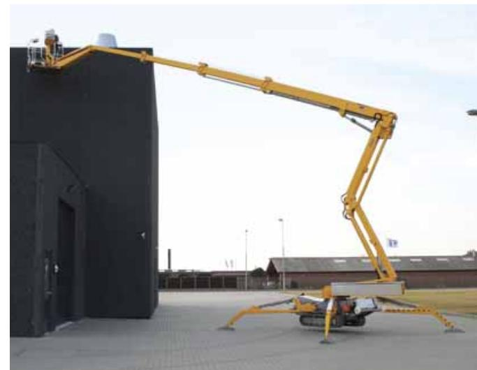
The 2500 RXBDJ also has impressive levelling ability and is able to climb and level up on slopes of up to 35 percent/19.3 degrees. With assistance to get into position it can level on slopes of up to 40 percent/21.8 degrees thanks to its high lift outriggers.
