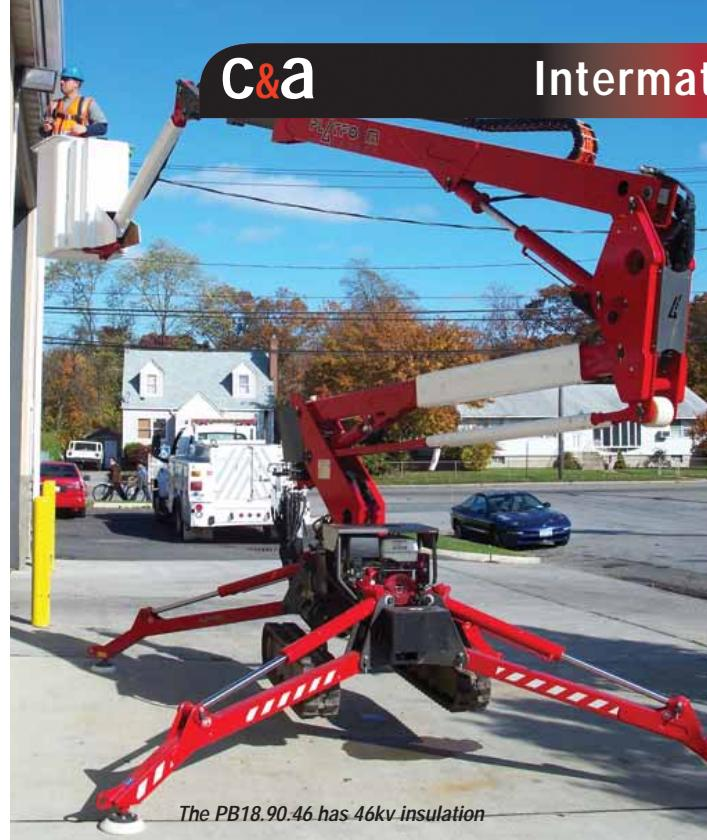
*The PB18.90.46 has 46kv insulation*
