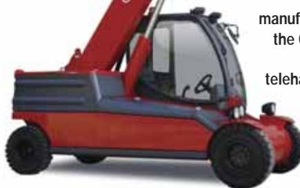
Italian pick & carry crane manufacturer Galizia has launched the GF60, a new six tonne crane based on its innovative telehandler/crane/platform Multis 636. The GF60 has a longer three section boom, with 7.5 metres under hook height.
