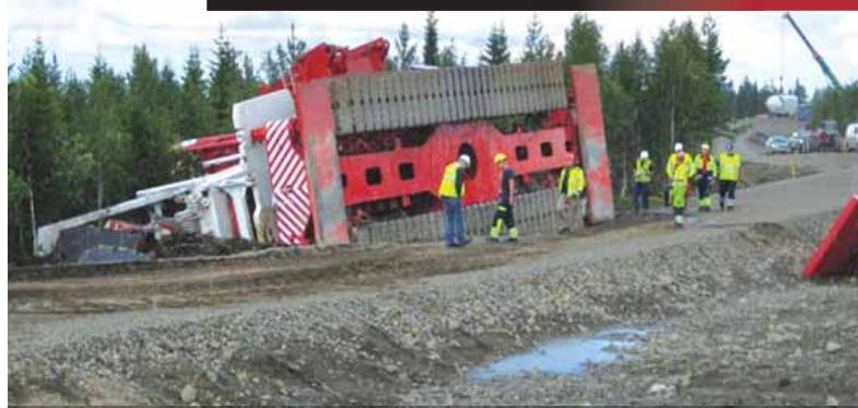
*Moving cranes fully or partially rigged can have disastrous results*
