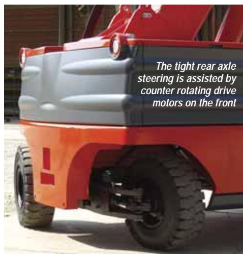
*The tight rear axle steering is assisted by counter rotating drive motors on the front*
