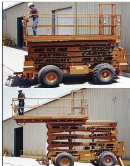
This rough terrain UpRight Flying Carpet of the early 70s has a platform height of 47ft with a 6ft hydraulic cantilever platform and a dual fuel petrol/propane system. Other features included a tow bar, 120psi and 120V power to the platform, spark arrestor exhaust system and foam filled tyres.
