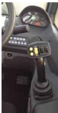
The single lever, electro-hydraulic joystick has been redesigned to include the 'up and down' transmission control buttons.
