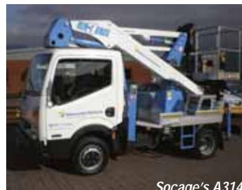
wheelbase Euro 5 Nissan Cabstar, the compact unit is ideal for street lighting, local authorities and city centres. Overall length is just 4.55 metres, travel height 2.65 metres and overall width 1.85 metres. With stabilisers deployed the machine has a footprint width of 2.3 metres which falls within the width of its wing mirrors.
