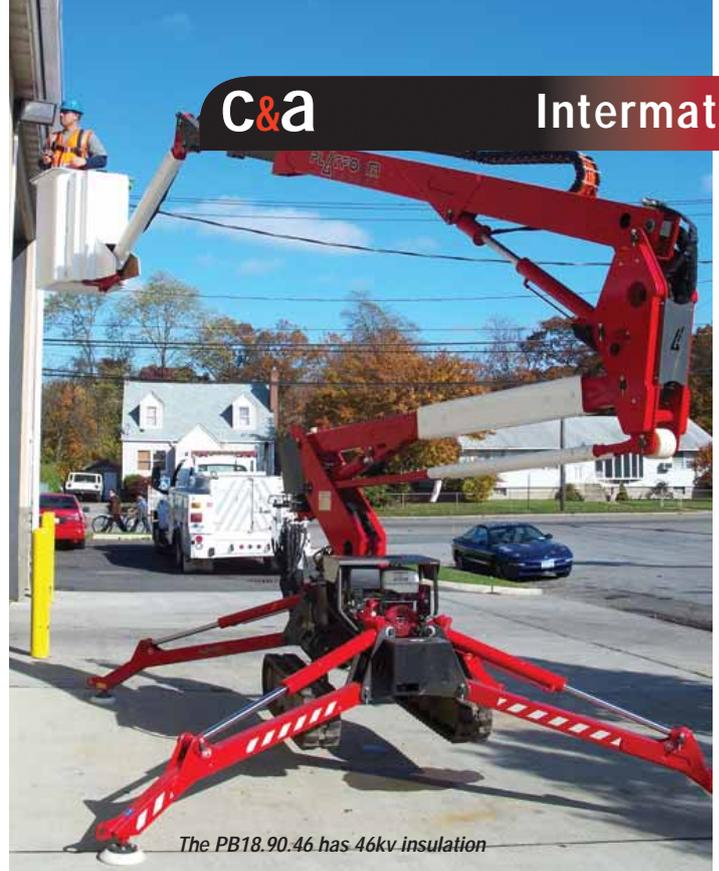
The PB18.90.46 has 46kv insulation
