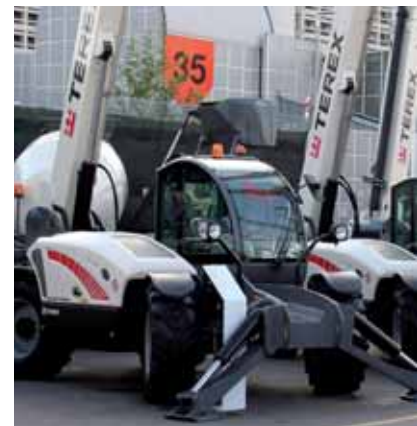
Terex showed its new 4013SX telehandler, a stripped down, lower cost unit with a mechanical gearbox, aimed at the rental market.
