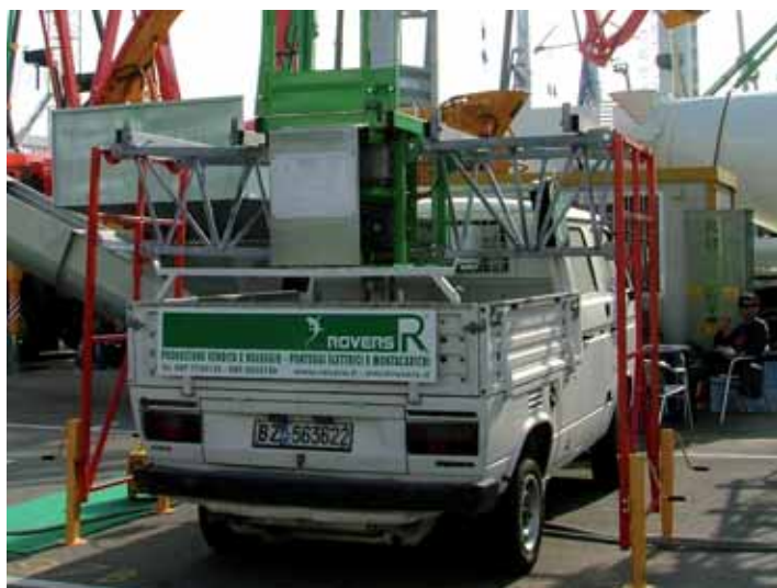
Rovers has designed a simple system for self unloading a mast climber base unit
