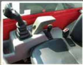
Joystick moves with operator's seat.
