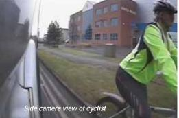
users find themselves in the blind spot of a large vehicle. So the company has fitted its entire truck fleet with a four point camera system which records the side and rear of the truck. It provides the driver with direct, real-time views from inside his cab as well as
