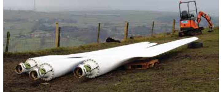
Each blade weighs 410kg
