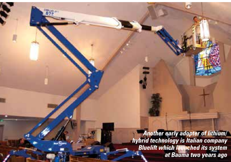
The Bluelift lithium battery system is also detachable so it can be moved from one unit to another, offering fleet owners greater flexibility
