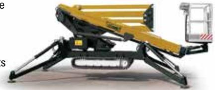
We begin the tour on the Teupen stand in outside area 5, to see its new 24 metre Leo 24GT which is based on the Leo 21GT, with its 12 metres of outreach, 250kg platform capacity and adjustable tracks. Also check its new Lithium-ion battery drive system.
