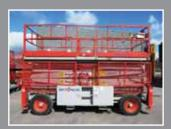
Skyjack SJ-9250 Diesel scissor lift 17.24m/909kg - 2007
