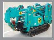
MAEDA MC 285 CRM Mini crane 8.70m/ 2.8 Tonne - 2006
