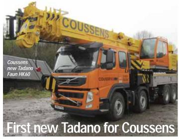
UK crane and access rental company Coussens of Bexhill has taken delivery of its first new Tadano Faun, a 60 tonne truck-mounted HK 60. The crane is mounted on a four axle Volvo FM commercial truck to allow it to carry more counterweight while keeping axle weights low enough to meet UK STGO Category B.
