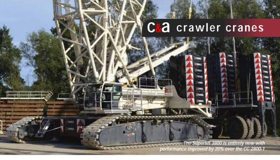
The superstructure can be equipped with the patented quick connection collar allowing it to be removed from the tracks in less than 30 minutes and weighs just 65.1 tonnes when stripped. None of the components exceed three metres wide by three metres high and all are less than 40 tonnes.
