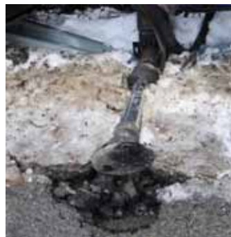
This incident was caused by putting the jack down with no spreader of any kind - in spite of its miniscule size
