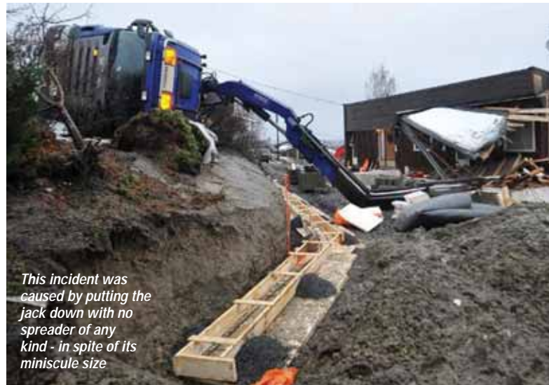
Outrigger incidents caused by structural failure are exceptionally rare
