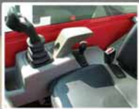
Joystick moves with operator's seat.
