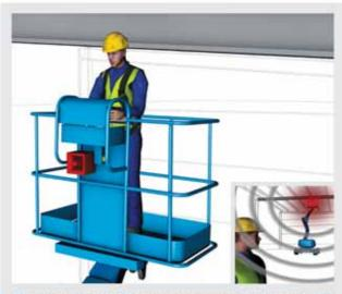
The pioneering SkySiren® is designed to simultaneously stop the movement of a machine in an entrapment situation, whilst also alerting colleagues to the incident with a flashing light and emergency siren.
