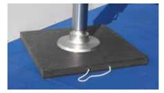
Reminder: Pad Size Calculator available from ALLMI. A template spreadsheet is available to help determine minimum stabiliser foot/pad size requirements
