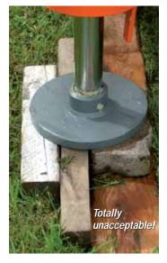
terrain by operators who are generally less experienced than those on larger cranes or platforms. On the other hand the very smallest cranes and lifts impose relatively low ground bearing pressures, with their standard fixed pads. They also tend to be a little more forgiving than larger equipment.
