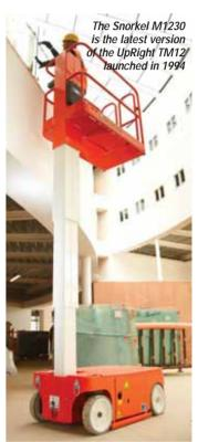
hotels and offices where the capacity is 680kg. Another benefit is the machine's compact dimensions - overall length of around 1.35 metres - again making them suitable for smaller elevators.
