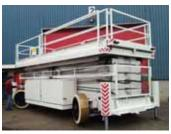
Holland Lift introduced a more compact version of is 34 metre working height electric scissor lift
