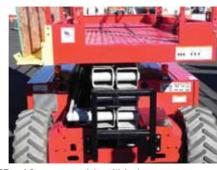
MEC offers an offset deck design on its ERT and Crossover models, which gives users a platform that extends to the full chassis width on one side and incorporates an inboard sheet or tube rack on the other side.
