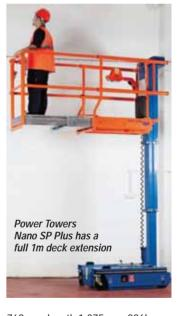
762mm, length 1,375mm, 226kg platform capacity and total weight of about 750kg. If there is a platform extension then it will be 500mm.
