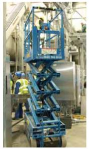
Most electric scissor lifts are slab models with seven to 11 metres working heights
