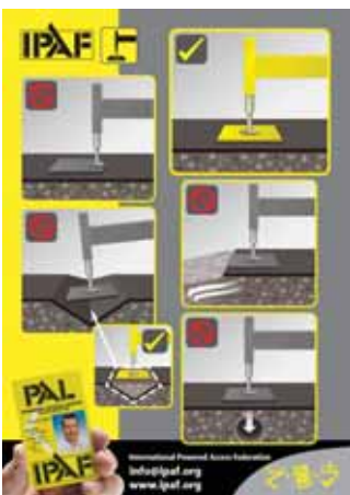
IPAF's "Spread the load" campaign calls for the proper assessment of ground conditions and the correct use of stabilisers, outriggers and spreader plates ( www.ipaf.org/spreaders )
