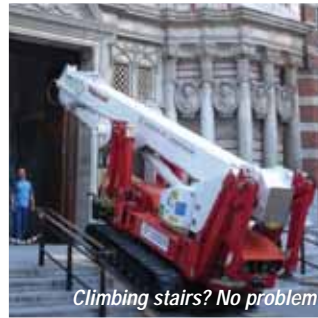
A Cela DT24 showing its gradeability
