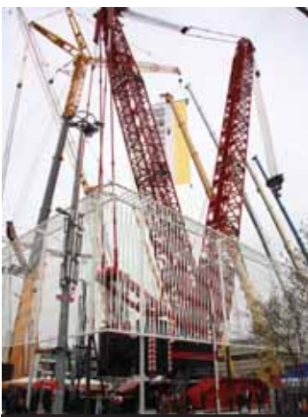
The 1,000 tonne LR 11000 slots between the 750 and 1350 tonne models having a 222 metre maximum lift height. Transportation is made easier with a maximum width of 3.5 metres and height of 3.2 metres with individual components. This was bought by Mammoet
