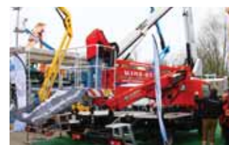
Isoli re-entered the large truck mounted market unveiling the 36 metre PTJJ 36.27 the first of a three model range with 48 and 60 metre models to come. Mounted on an 18 tonne chassis it has 27 metres outreach
