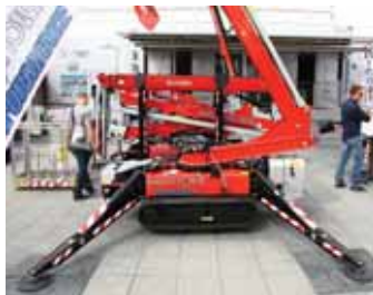
Hinowa 20 metre Lightlift 20.10 Performance IIIS with lithium battery or new diesel engine
