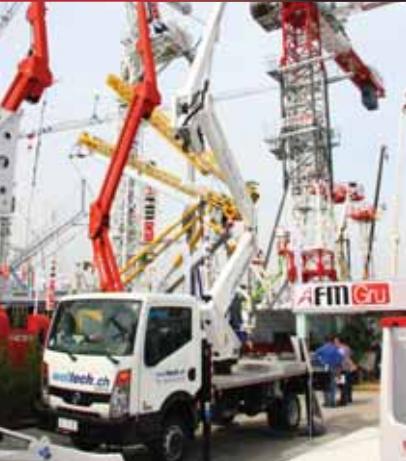
Lots to see on the CTE stand including the Zed 20.2 HV with variable outrigger positions, 300kg maximum basket capacity and full 9.2 metre outreach narrow jacked with 120kg in the basket
