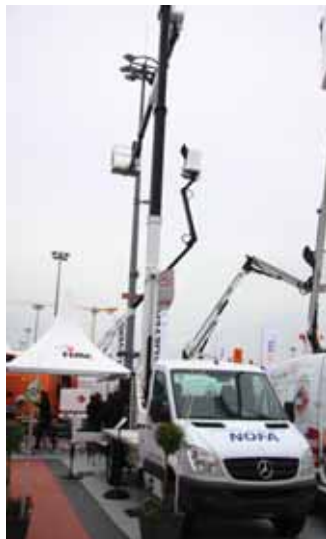
One of many interesting new products from Versalift the 24.5 metre working height VTX 240 mounted on a 3.5 tonne chassis
