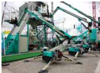
Imer has its range of three spiders including the IM R13 spider - a light and compact platform with three telescopic extension and jib
