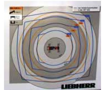
The variable supporting base from Liebherr prevents the operator from accidentally or deliberately fooling the Liccon - LMI - with regard to outrigger position or ballast configuration
