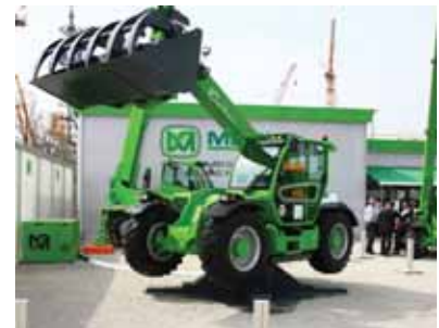
Merlo launched its five tonne Panoramic 50.8 and its four tonne Roto 40.18S which offers an 11 metre lift height at full capacity
