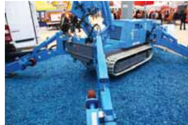
R&B showed a new one tonne capacity CR174GE previously a 1.7 tonne capacity crane but has been reduced for CE certification. The CR335D now has a new fly jib and searcher hook and 500kg pick and carry capacity using these foldaway wheels
