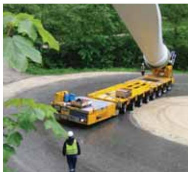
The 45.6 metre long blades were elevated up to 60 degrees to negotiate the narrow turns on the mountain roads.
