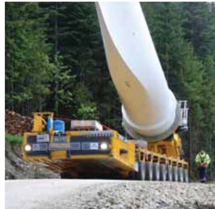
The 45.6 metre long blades were elevated up to 60 degrees to negotiate the narrow turns on the mountain roads.
