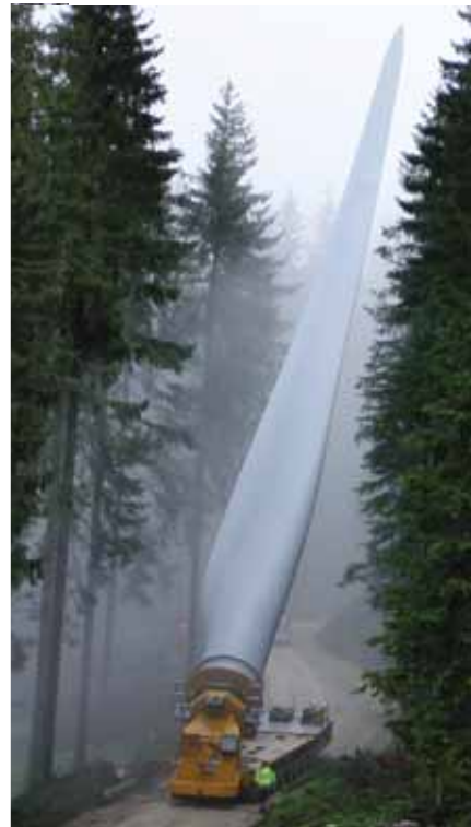
The 45.6 metre long blades were elevated up to 60 degrees to negotiate the narrow turns on the mountain roads.
