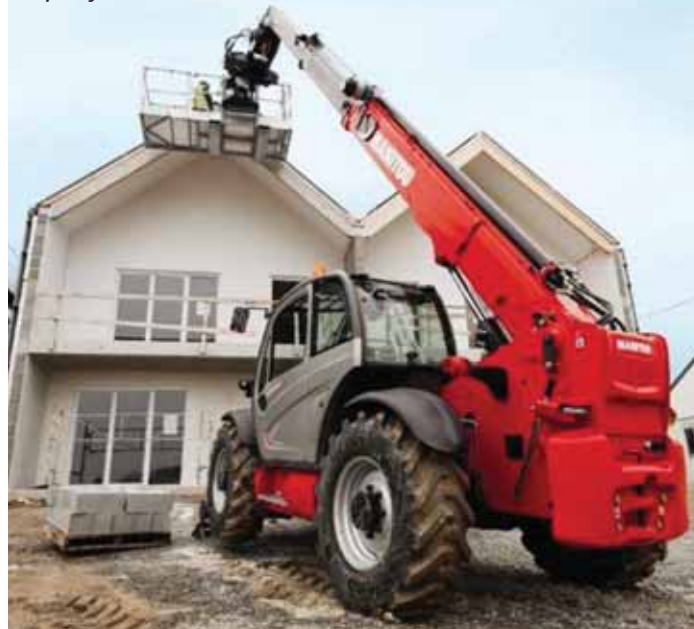
Manitou has three all new models - the eight metre MT 835, 11 metre MT 1135 and the 13 metre MT 1335 (below) - are rated at 3.5 tonnes lift capacity and share a common chassis
