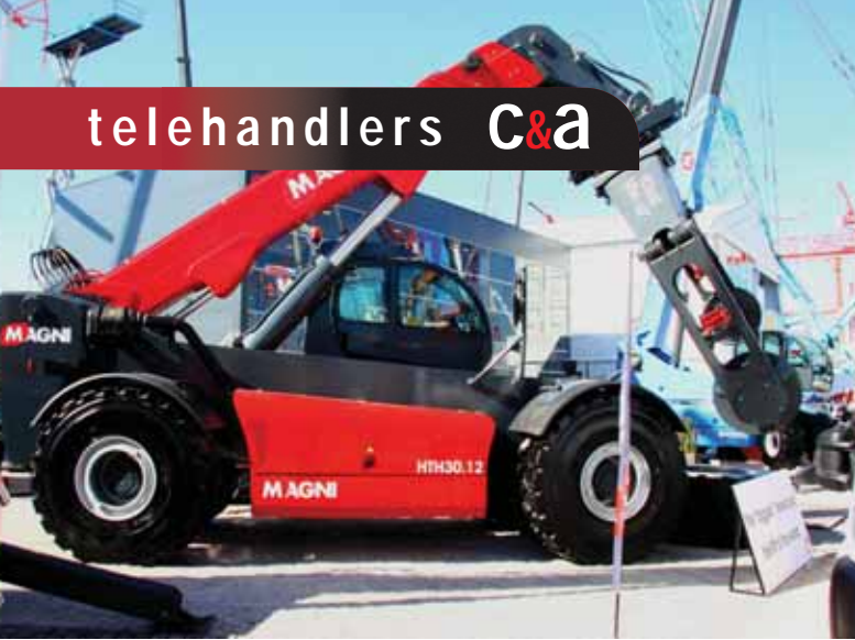
The Magni HTH 30.12 claims to be the biggest telehandler in the world with a 30 tonnes maximum capacity and 11.7 metre maximum lift height
