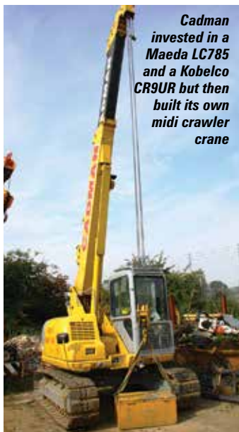
Maximum capacity of the ACC 2050 on the main boom is 8.9 tonnes at a radius of 4.6 metres, 2,170kg at 16.2 metres and 1,120kg at 22.8 metres (ACC 2050/2)
