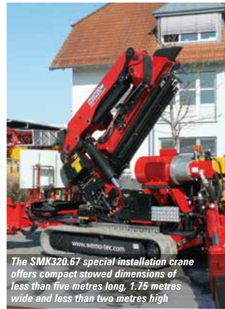
The SMK320 was also fitted with a four axis manipulator arm integrated into the boom design
