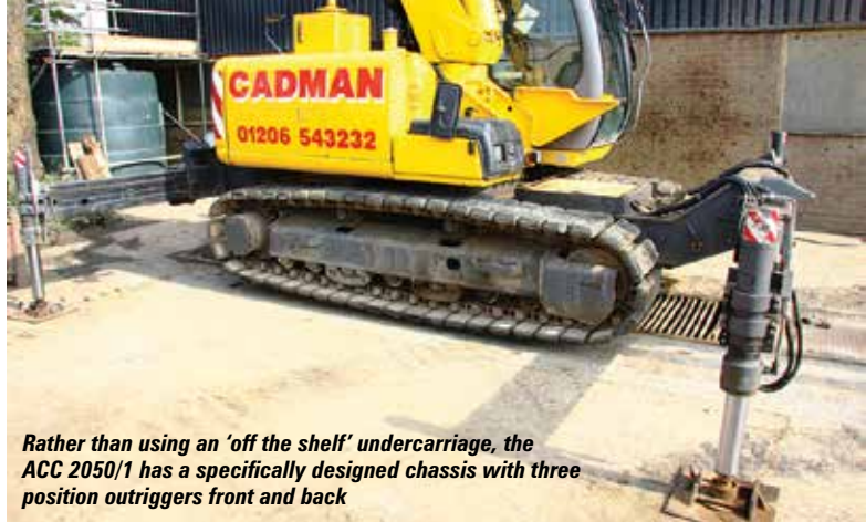
Cadman designed its own mid-sized crawler crane with articulated telescopic boom
