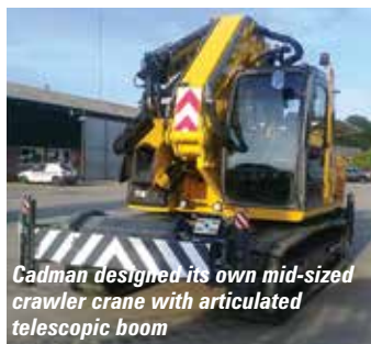
Rather than using an 'off the shelf' undercarriage, the ACC 2050/1 has a specifically designed chassis with three position outriggers front and back
