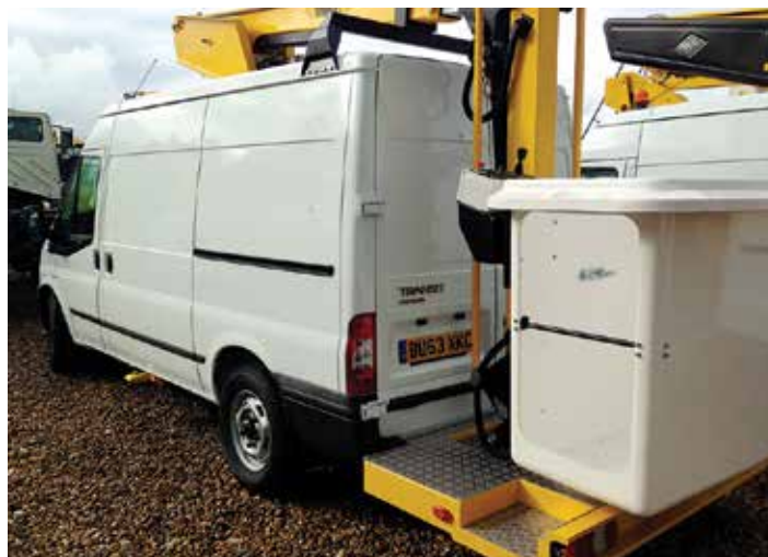
Versalift has adopted the same under-run method as its sister company Time Export (Denmark) in order to comply with specific legislation
