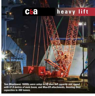
boosting their capacities to 400 tonnes. The deckhouse was rigged with 12 nylon straps and then lifted from the barge to a height of 27 metres and held in place for three hours, while the barge was moved out from underneath and the 12,000 tonne ship was moved into place underneath, allowing the deckhouse to be lowered onto the ship's hull. Contractor Reed & Reed provided
