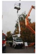
The GSR E140P mounted on a Piaggio compact chassis
