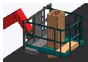
The device's folding platform and guardrails can then be closed completely encircling the structure
