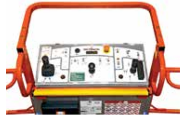
The Skyjack SG-E secondary guarding system
