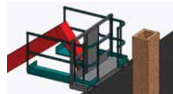
Once positioned against a vertical structure the platform's hydraulic sides can be adjusted
