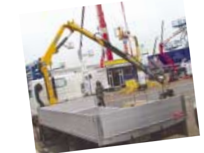
Effer showed its Easy power 30 for a 3.5 tonne truck with 7.8m outreach
